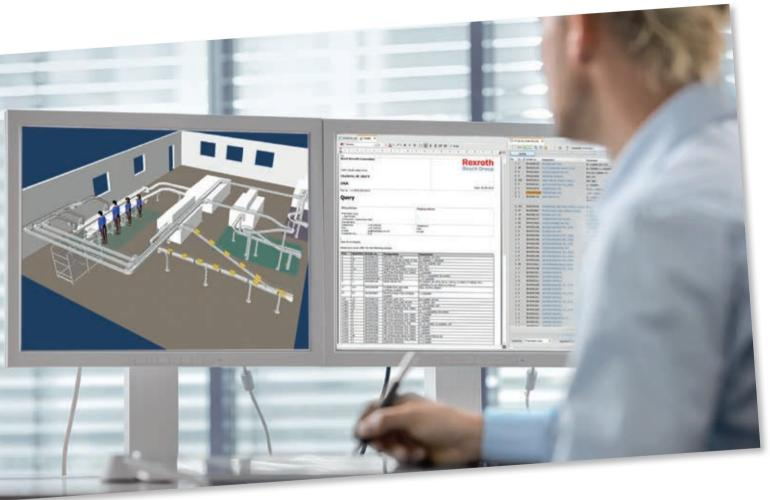
MT*pro* is an intuitive piece of software used for planning assembly systems. It assists you from selection and configuration through to ordering components.
